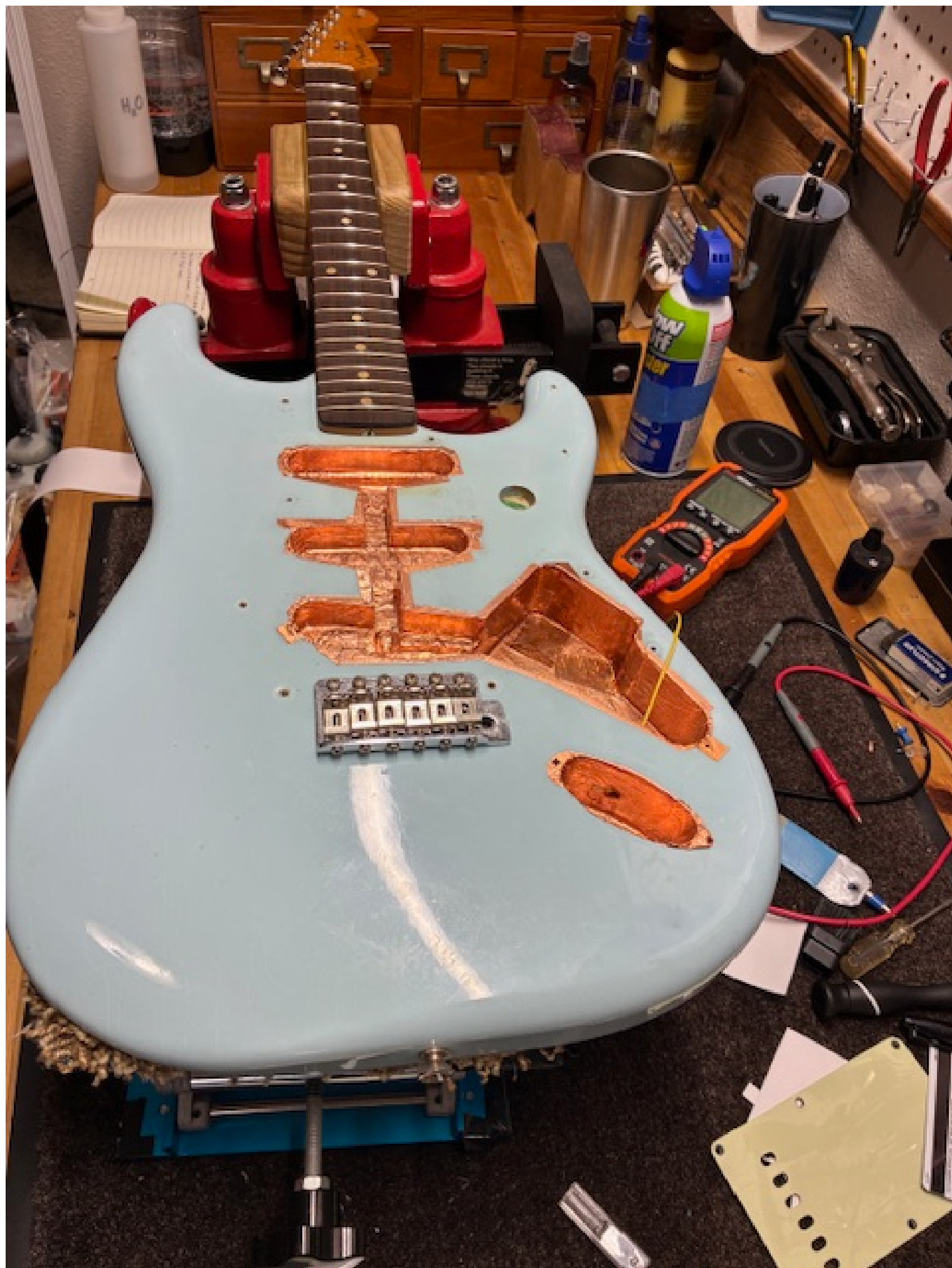
Fully shielded Stratocaster with conductive copper tape
