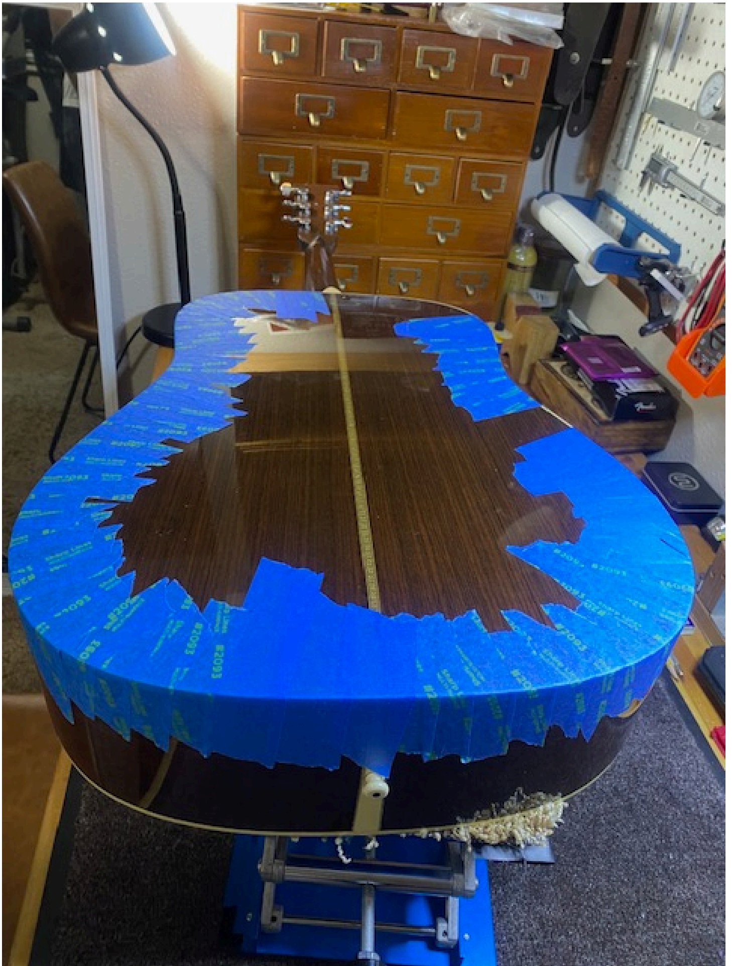
Martin D28 binding repair no.2
